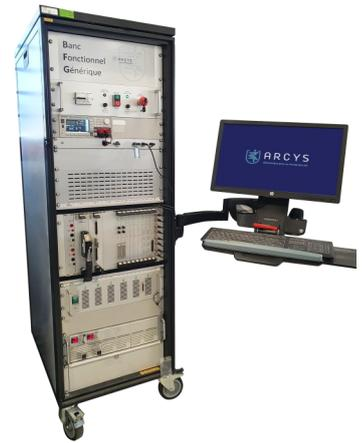
The Generic Functional Bench (BFG) allows different test modes to be carried out on several types of products with a minimum of adaptation. It authorizes the running of a set of scenarios that will sanction the compliance and performance of the equipment under test. Its "step by step" mode allows rapid fault diagnosis during the PRODUCTION or after-sales service phases of the equipment under test. A self-test and an automatic calibration facilitate its periodic maintenance.
